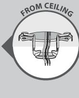
CONNECT WIRES FROM RECEIVER AND FAN TO WIRES FROM OUTLET BOX - Using the orange wire connectors, connect the black wire (ungrounded) from the ceiling to the black wire from the receiver. Connect the white wire (grounded) from the ceiling to both the white wire from the receiver and the white wire from the fan.
